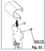
4. Orient the rod correctly and fit the safety screw.
