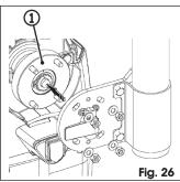
Check if the rod is perfectly vertical and secure the four nuts.
